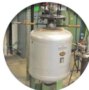
Head Treatment (hardening and tempering)
